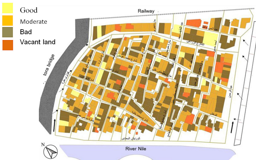
Figure 7: Building condition of Tora
