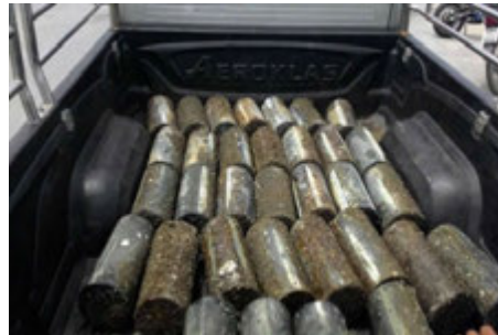
Figure 2: Concrete specimens soaked for 90 days under marine environment.
