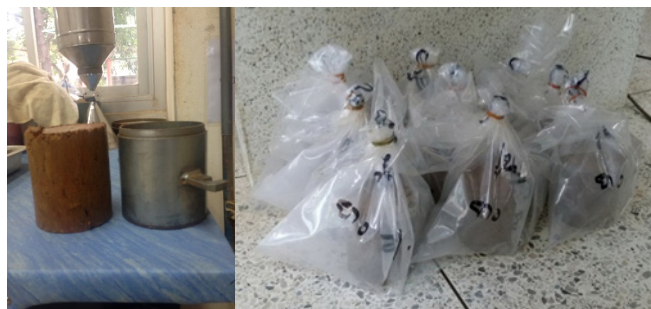
Figure 3: trial batch demonstration specimens and curing
