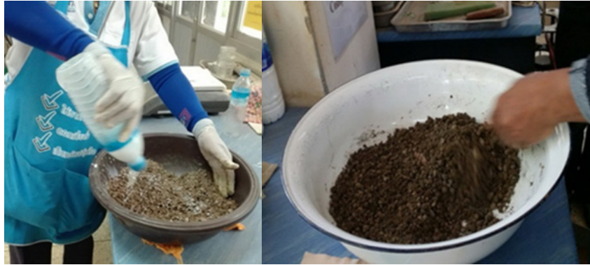
Figure 2: A trial batch demonstration showing a mix together of soil, cement, water, surfactant and NRL liquid.
