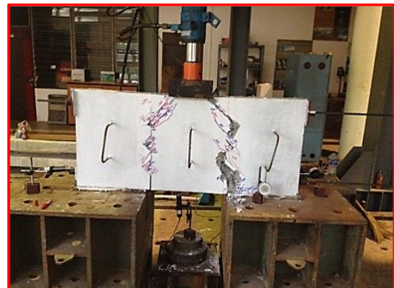
Figure 5: Shear test of multiple key triangle shape stressing 0.833 MPa
