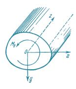
Figure1: Anisotropic cylinder
