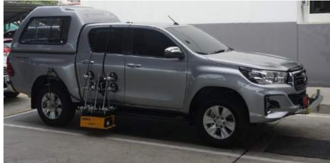
Figure 4: the pickup truck used for measurement of IRI in this research.
