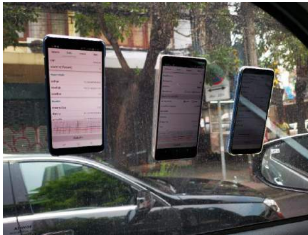
Figure 3: Installation of the mobile phones adhered to the window of the pickup truck.
