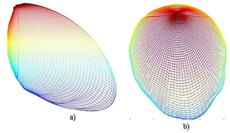
**Figure 5:** The estimated PB of a system of two differently oriented radiators: a) in a vertical plane C90-270; b) in the horizontal plane
