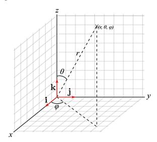
Figure 1: Angular coordinates in a spherical system
