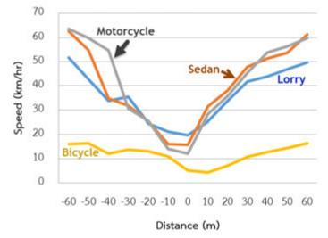
Figure 4: 85<sup>th</sup> percentile speeds passing through used tires of six-wheel lorry.
