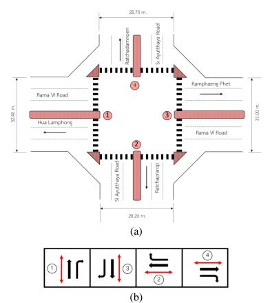
Figure 2: Physical and traffic signal phase of the Sri Ayutthaya intersection.
