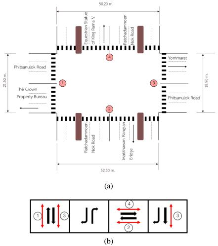
Figure 4: Physical and traffic signal phase of the Suan Miskawan intersection.
