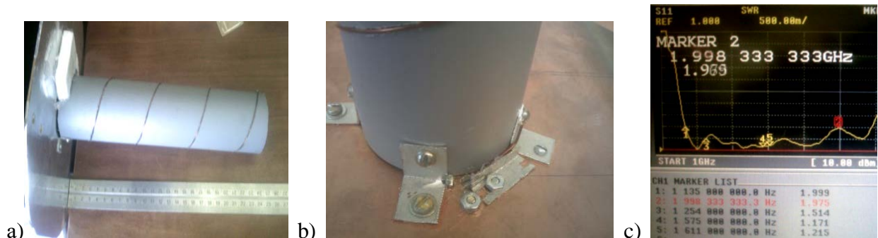
Figure 4: The multi-band antenna for the stroboscopic test unit to measure the radiation pattern: a) The antenna with winding for operation with circular polarization; b) A method for tuning the antenna; c) The voltage standing wave ratio (VSWR) for the antenna.
