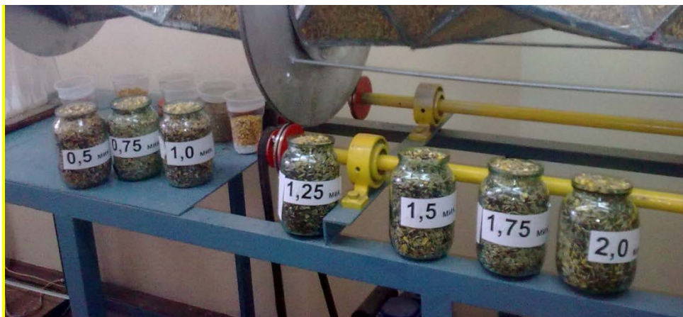
Figure 6: Samples of the feed mixture after conducting research on the process of mixing them in the RC 5.1.a relational screw drum for 0.5-2.75 min.
