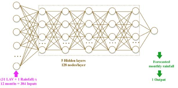
Figure 2: DNN architecture developed with 384 inputs to predict the monthly rainfall forecast.
