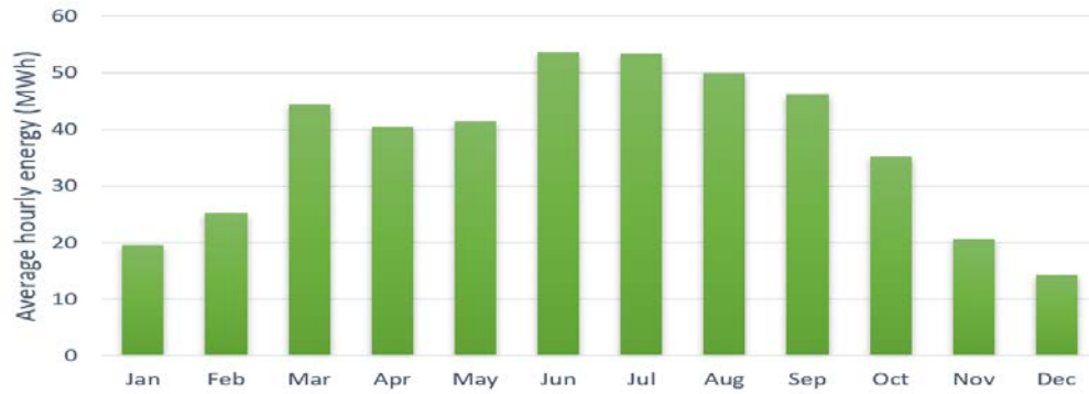
Figure 7: Hourly average energy of CSP plant.
