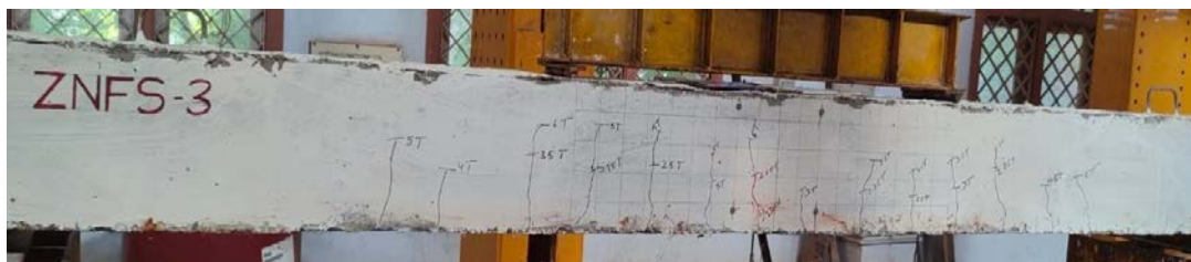
(f) Crack Pattern of ZNFS-3
