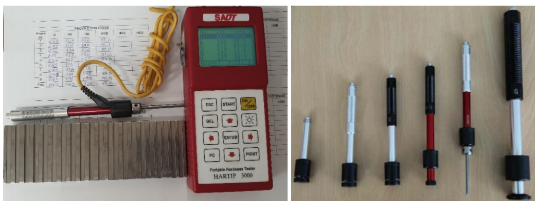
Figure 1: Portable hardness tester HARTIP 3000.
