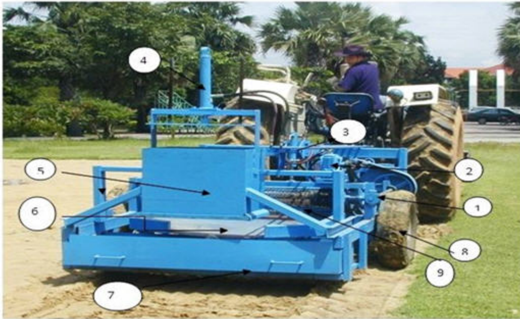
Figure 3: .Beach cleaning trailer prototype 1.cam 2. Gear box 3. Front hydraulic cylinder 4. Rear hydraulic cylinder 5. Hydraulic compressing unit 6. Shaking sand tray 7. Trash tray 8. Wheel 9. Transporting system
