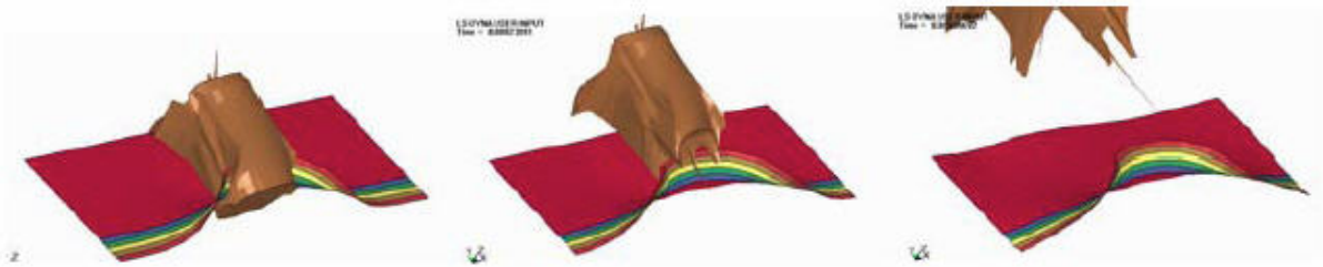
Figure 16: Snapshots of the a bird impacting the tapered plate at 30°.
