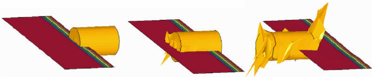
Figure 20: Snapshots of the a bird impacting the tapered plate at 0^\circ when using *MAT NULL.
