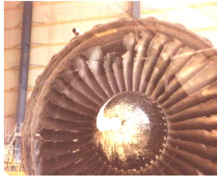
Figure 8: Damage caused by bird-strikes.
