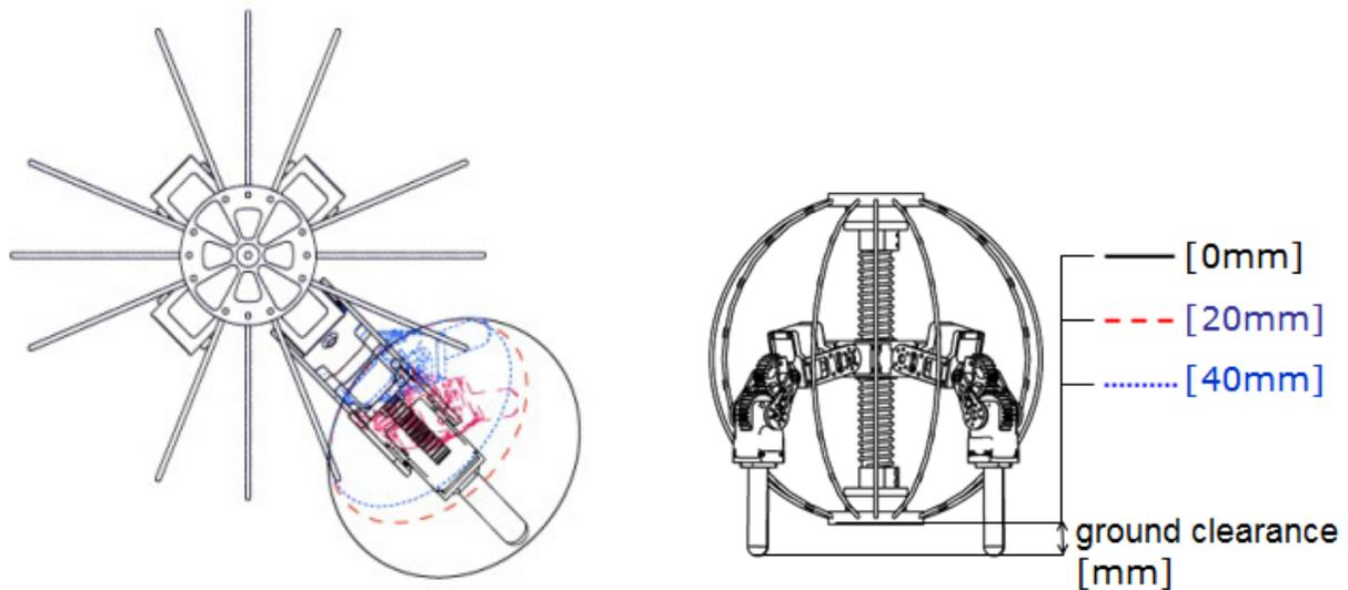
**Figure 11:** Results of paths of leg's end point.
