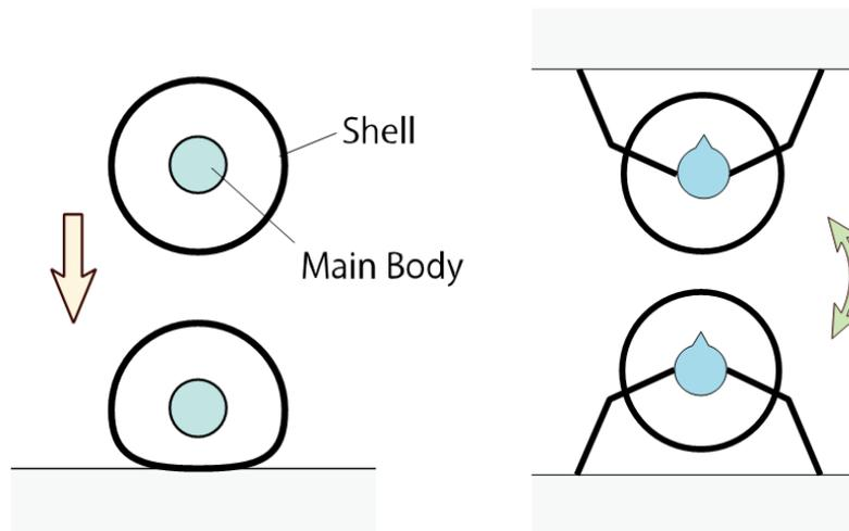
**Figure 2:** Spherical shell for shock-proofing.
