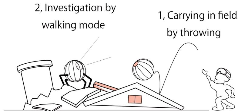
**Figure 1:** Application concept of our robot
