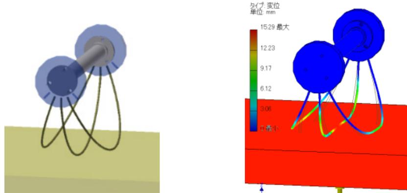
Load is acted in front of a wire of the spherical outer shell
