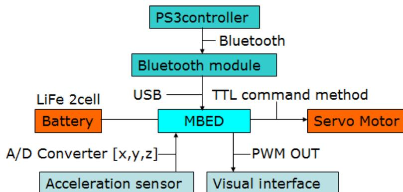
**Figure 12:** System configuration of prototype model.
