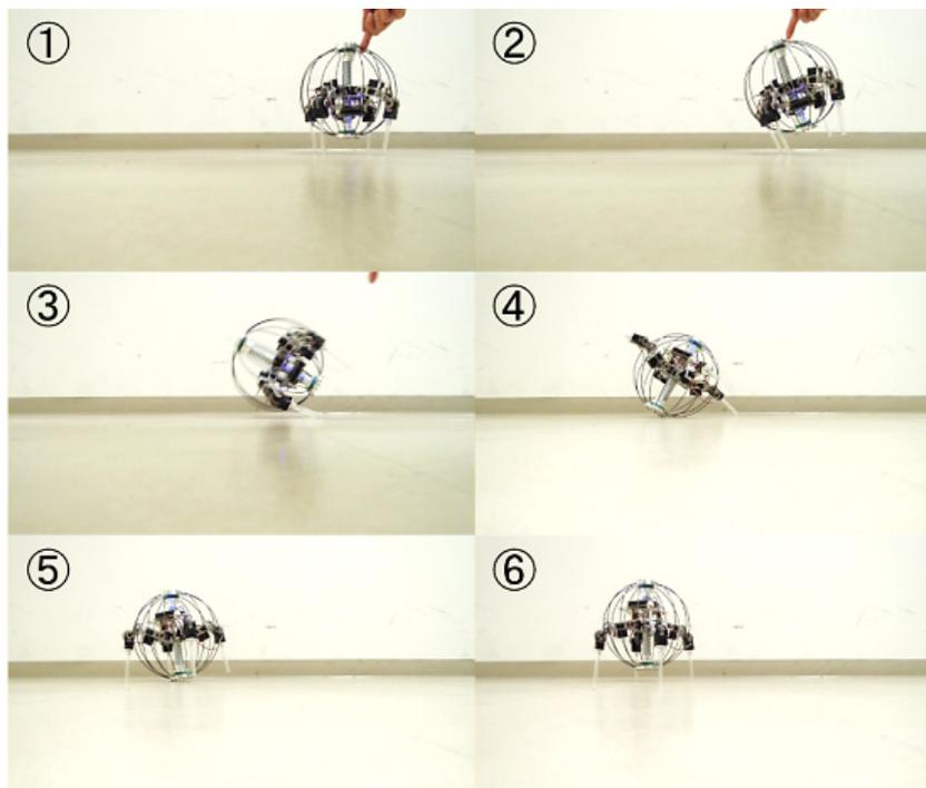
**Figure 16:** Return from fall state by autonomous system.
