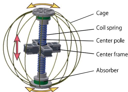
**Figure 4:** Structure of spherical shell of QRoSS.
