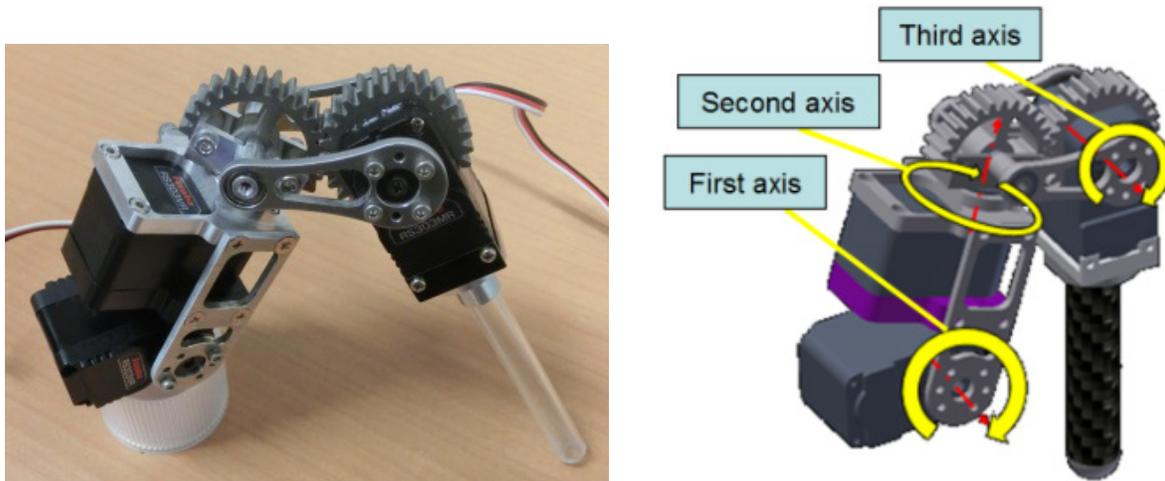
**Figure 9:** Prototype model of leg module.
