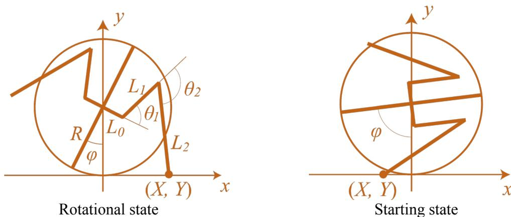
**Figure 13:** Two-dimensional model of QRoSS
