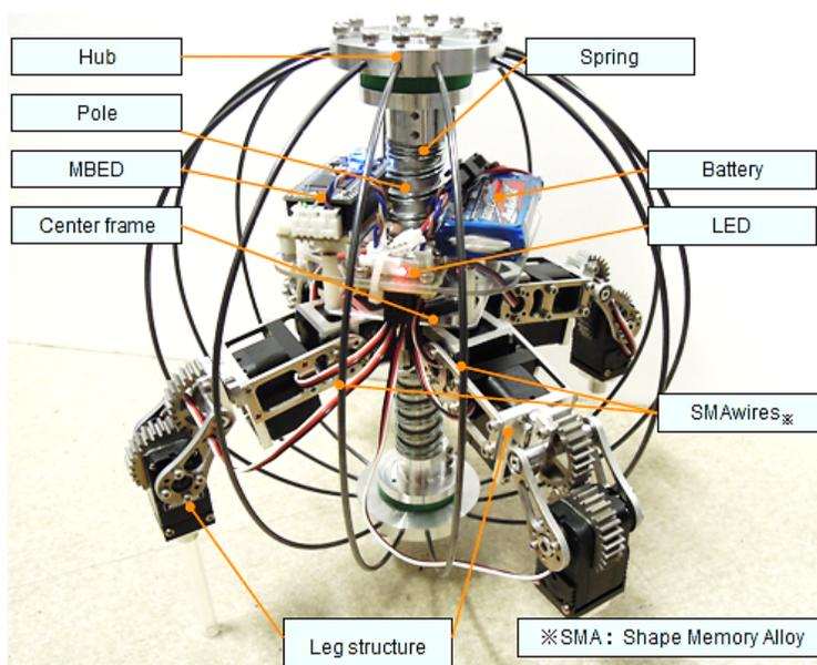
**Figure 7:** First prototype model of QRoSS.
