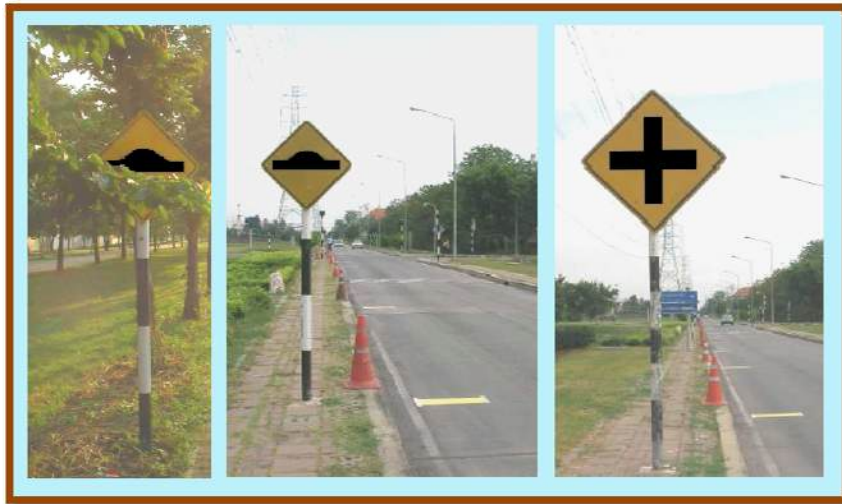
Figure 5: Bump (hump) and crossroad signs.
