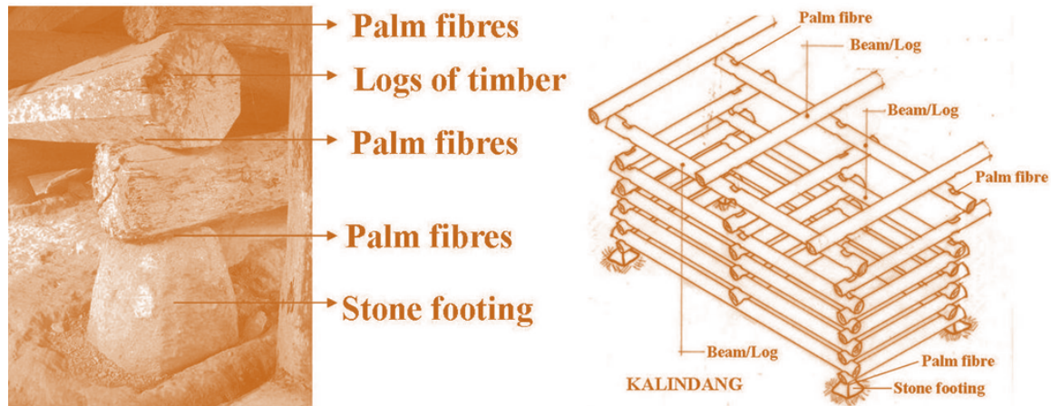
Figure 7: The lower structure of lamban tuha ( kalindang and stone footings)
