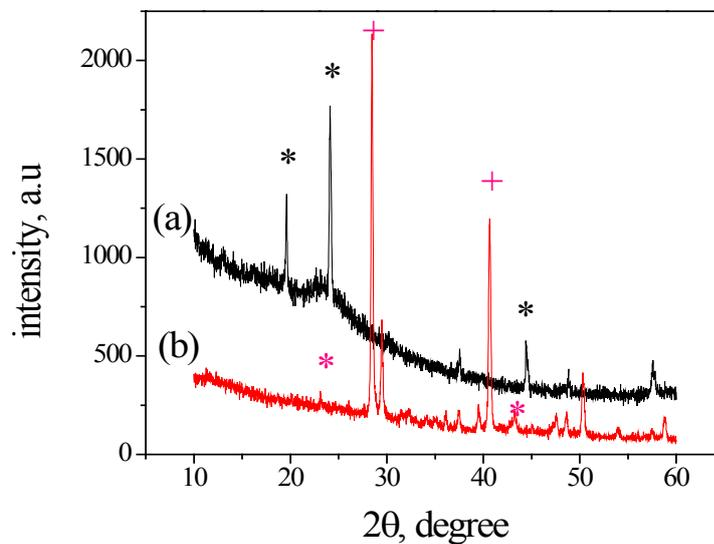
**Figure 2:** XRD spectrogram of (a) commercial activated carbon (Ciba) was added for clarify reading and (b) WH carbon, (\* = Carbon, ICDD no. 41-1487; + = KCl (Sylvite), ICDD no. 64-0312; others would be considerable as SiO<sub>2</sub>, Al<sub>2</sub>O<sub>3</sub>, and CaO especially for WH carbon )
