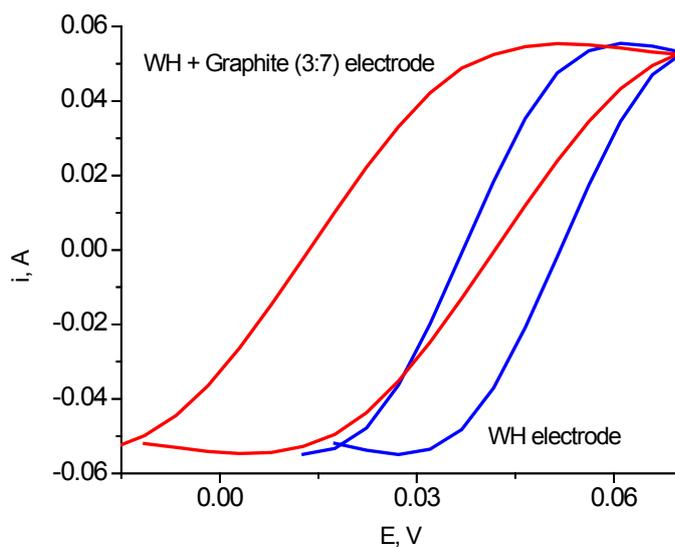
**Figure 6:** Voltammogram of water hyacinth (WH) carbon and WH + graphite electrodes in  $K_2C_2O_4$  1M. WH and WH + graphite electrodes were made from the mixtures of the materials and epoxy resin, respectively.
