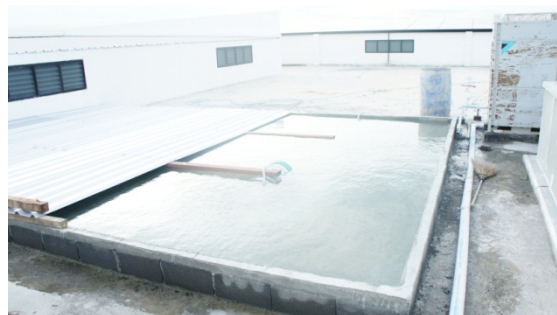
Figure 4: Loading by Water.
