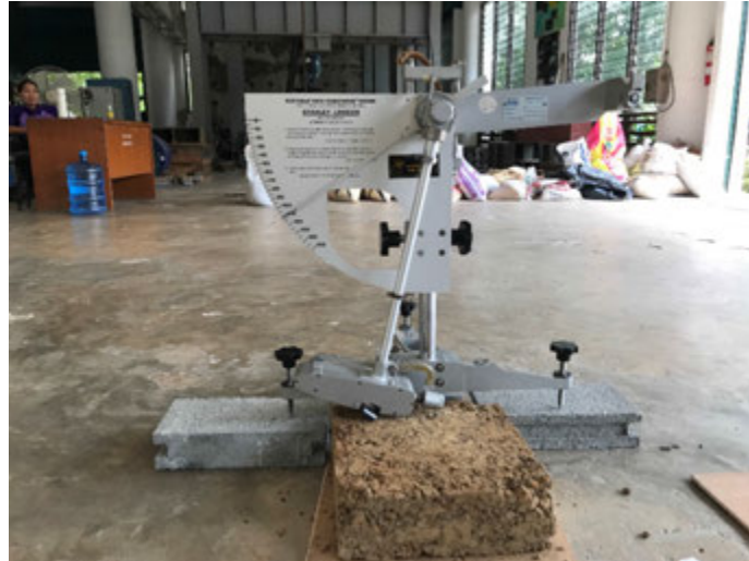
Figure 5: Portable Skid Resistance Tester (British Pendulum Tester (BPT)) of a trial batch demonstration specimen from the mix of natural rubber latex soil cement
