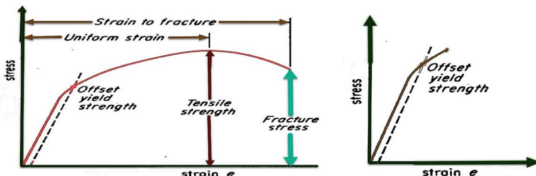
Figure 1: Stress-strain curves for ductile and brittle materials.
