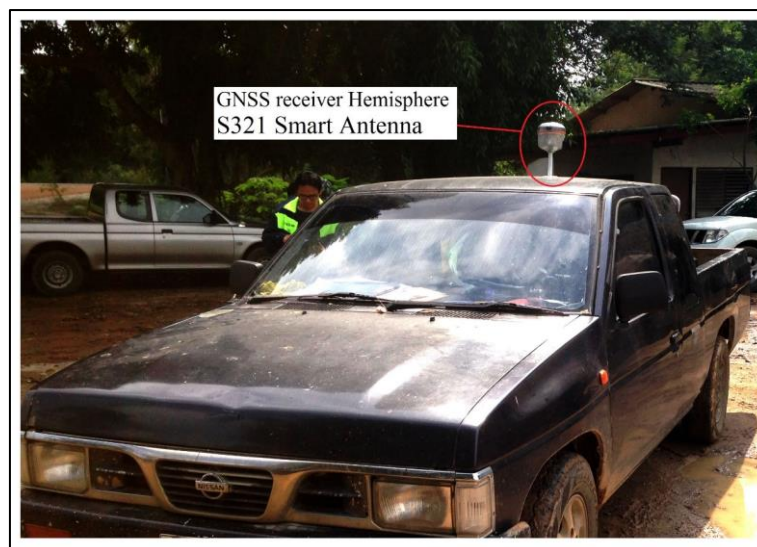
Figure 2: HEMISPHERE S321GNSS RECEIVER on top of the off-road car
