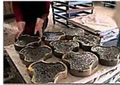
Figure 6: Setting the pavers.
