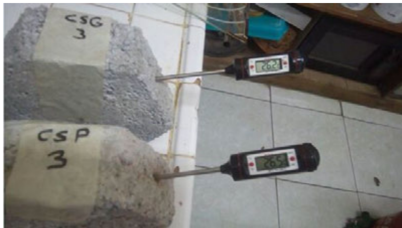
Figure 2: Temperature measurement inside the paver samples.
