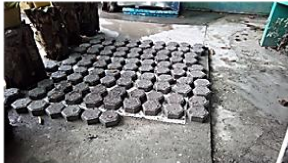
Figure 7: Taking pavers from the mould.
