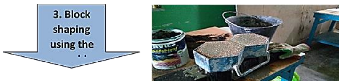
Figure 5: Putting the mixed materials into paver mould.
