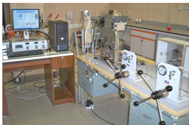
Figure 1: IFT Experimental set up using Pendant drop technique
