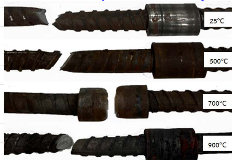
Figure 9: The reinforced steel with parallel thread mechanical splicing (PTC) failure mechanism after being heated with various temperature
