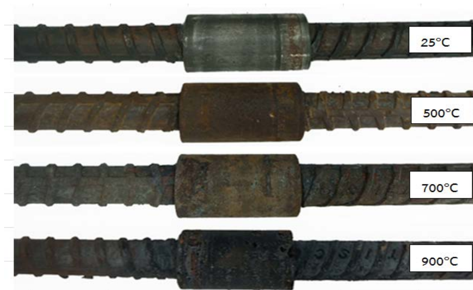
Figure 8: The reinforced steel with parallel thread mechanical splicing (PTC) failure surface after being heated with various temperature
