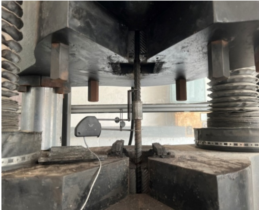
Figure 4: Monotonic tensile strength testing.
