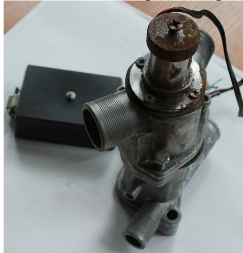
Figure 1: Electric regulator with solid filler and EH.
