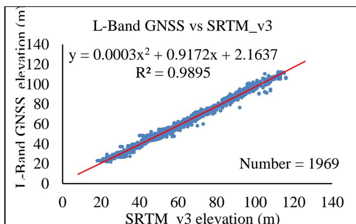
**Figure 6:** Vertical comparison between GNSS data with SRTM
