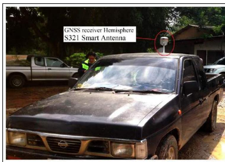
Figure 2: HEMISPHERE S321GNSS RECEIVER on top of the off-road car
