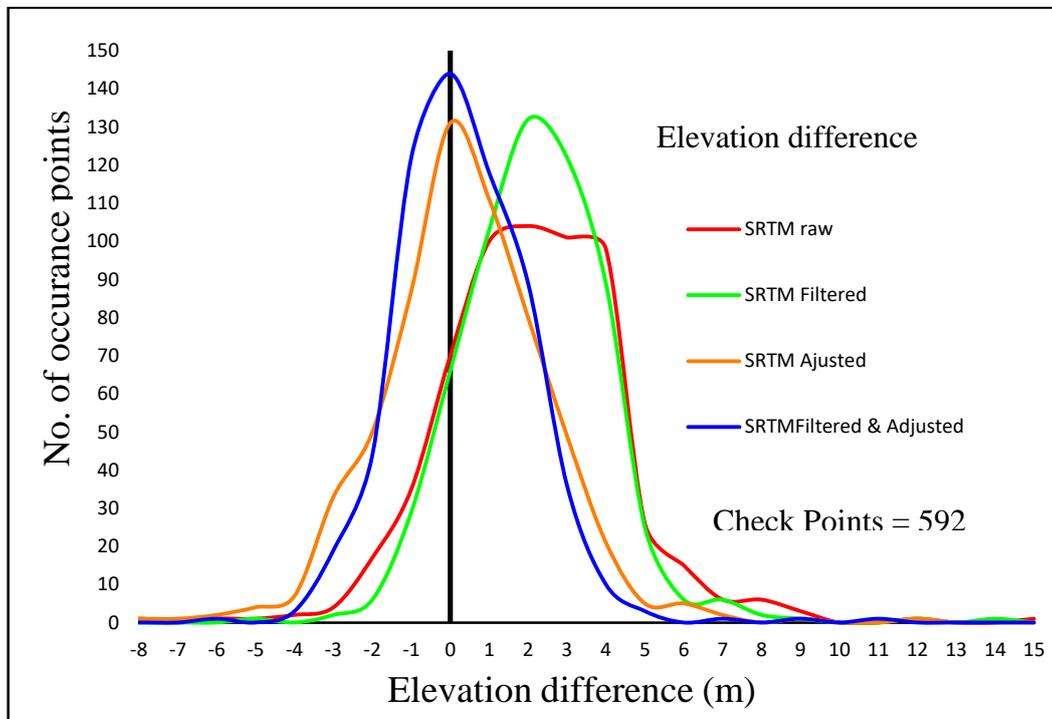
**Figure 8:** The histograms of elevation differences of the final accuracy assessment
