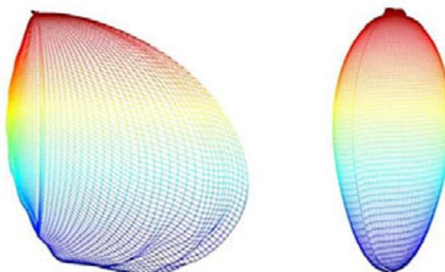
**Figure 3:** Photometric bodies of sources 1 and 2, obtained from the measurements
