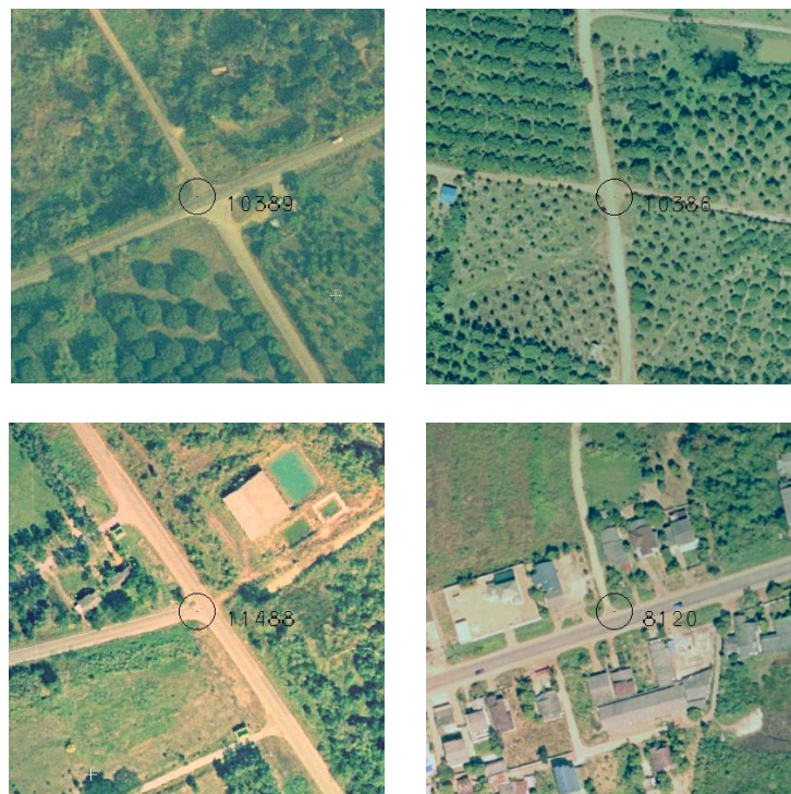
Figure 7: Examples of checkpoint locations, often at road intersections.
