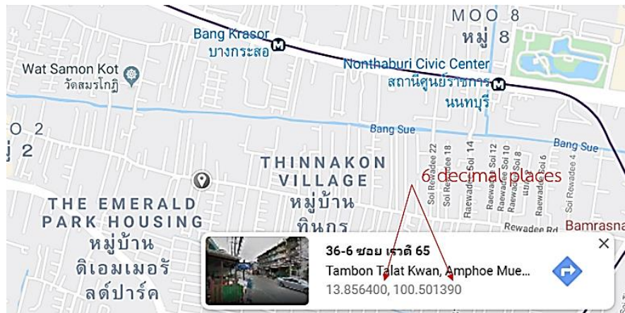
Figure 1 Google Maps displaying geographic coordinates with a precision of 6 decimal places or 0.1 meters. (Courtesy of Google).
