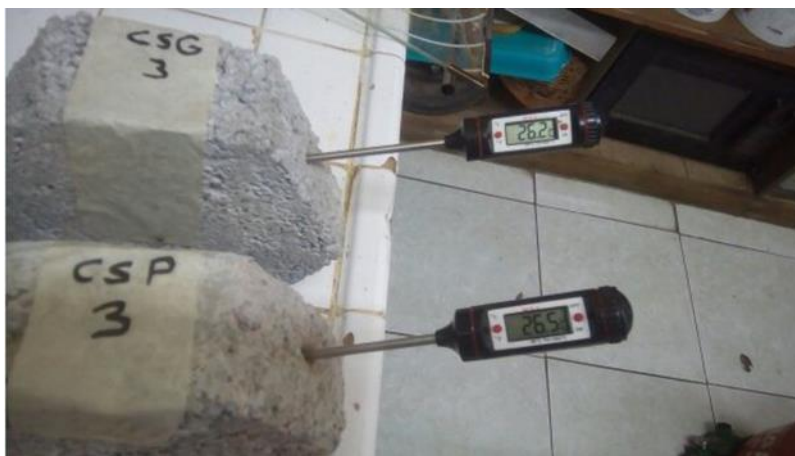
Figure 2: Temperature measurement inside the paver samples.
