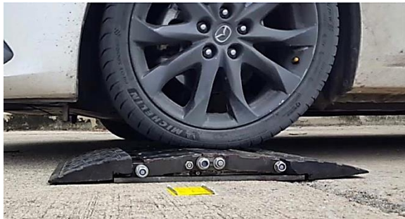
Figure 13: Fold-flat at 6 km/hr.
