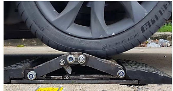
Figure 14: Locking at 12 km/hr.
