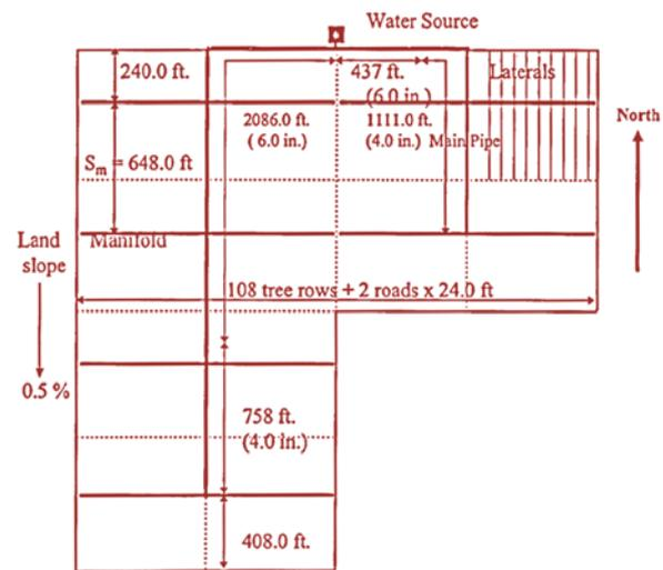
**Figure 6a:** Model design for farm layout and main pipe network (laterals are 16 mm PE, manifolds are SDR 26 PVC, and main lines are SDR 41 PVC).
