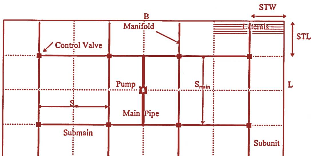
Figure 1: Configuration [1] for Trickle Irrigation Systems.
