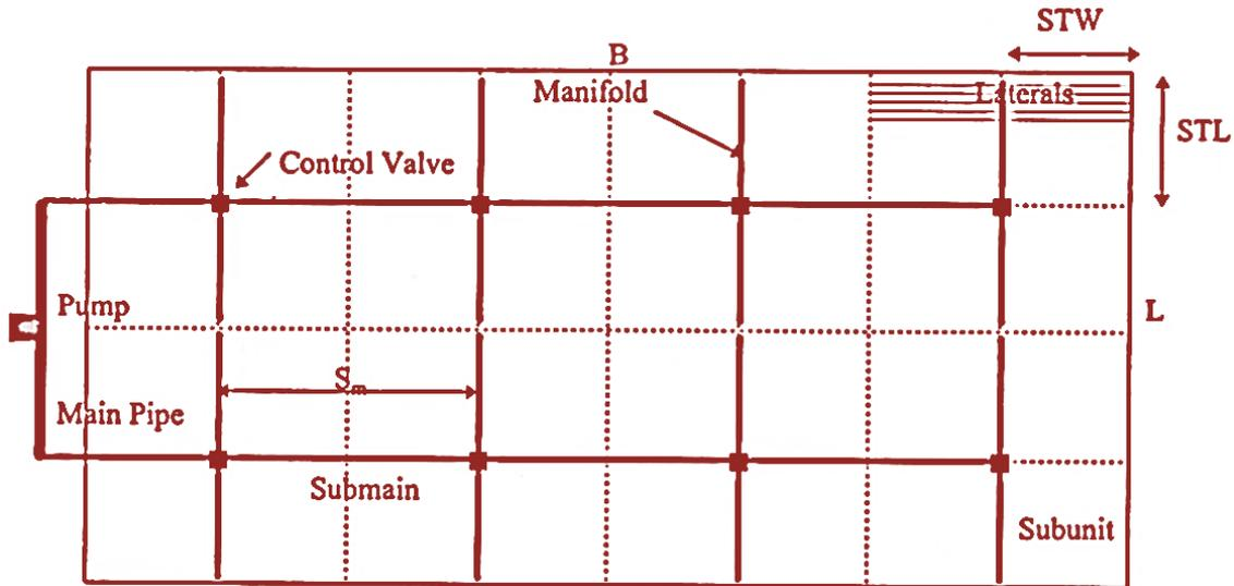
**Figure 2:** Configuration [2] for Trickle Irrigation Systems.
