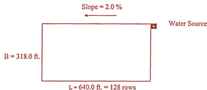
**Figure 4:** Tomato Field with Line-Source Drip Irrigation System [Keller and Bliesner, 1990].
