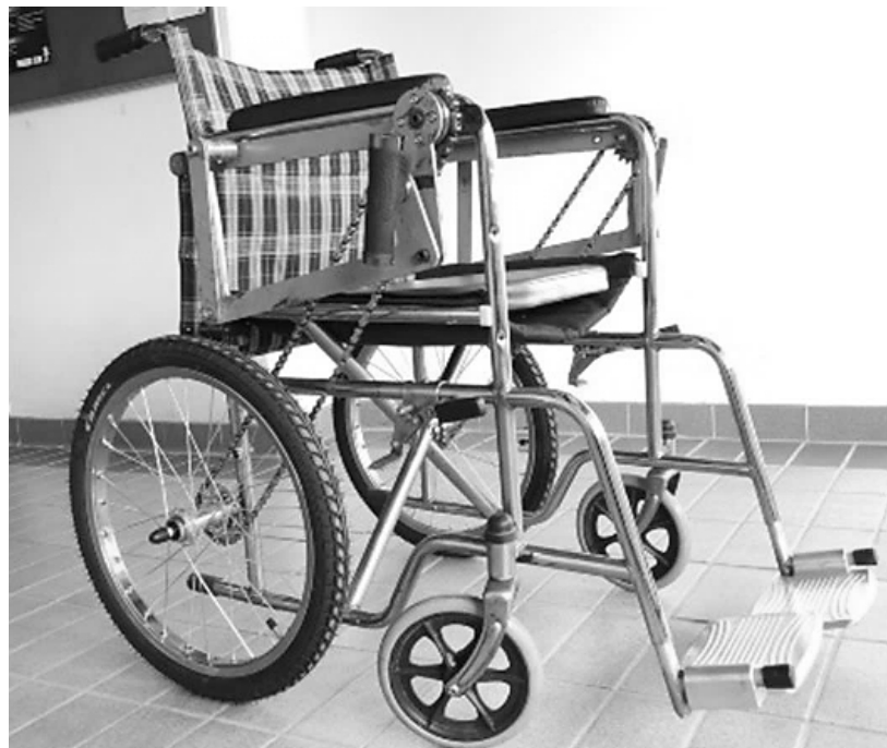
Figure 7: Prototype with EEF propulsion mechanisms on both sides of a conventional push-rim wheelchair.
