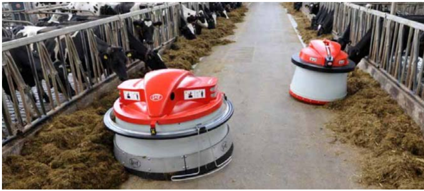
Figure 4: LELY JUNO Automatic feed pusher (Courtesy of Lely.com).
