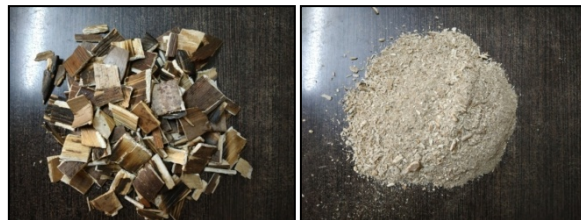
Figure 13: Dry, Compact and Torched (35seconds grinding time).
