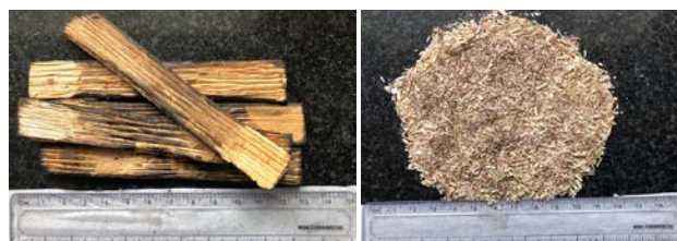
Figure 6: Dry, Compact and Torched (40seconds grinding time).
