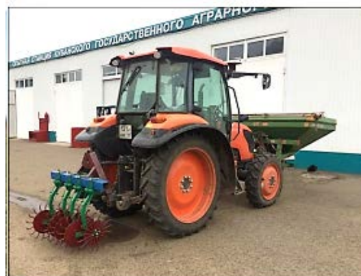
b) general view of the unit for harrowing crops with a rotary hoe with simultaneous top dressing
