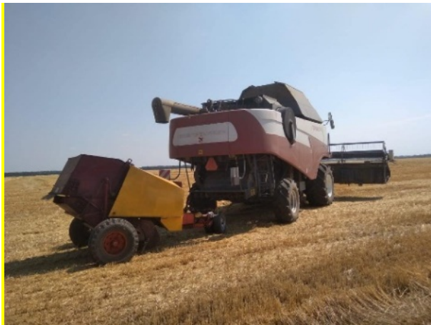
Figure 5: General view of the multifunctional harvesting unit with the simultaneous pressing of straw (a) and a graph of the dependence of the cost function C_c and loss C_1 (b)
