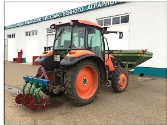
b) general view of the unit for harrowing crops with a rotary hoe with simultaneous top dressing
