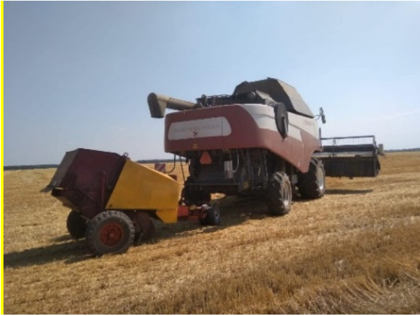
Figure 5: General view of the multifunctional harvesting unit with the simultaneous pressing of straw (a) and a graph of the dependence of the cost function C_c and loss C_l (b)
