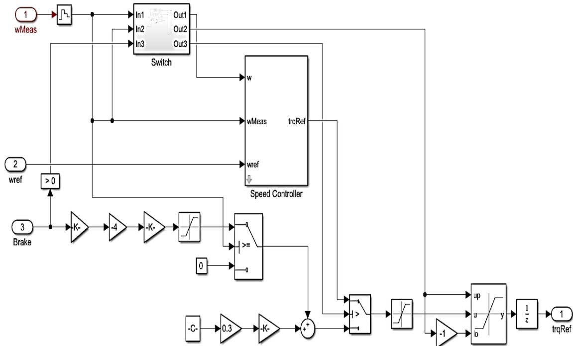
**Figure 5:** Simulink Model for Vehicle speed controller.
