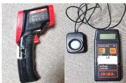
Figure 3: Infrared Thermometer & Lux Meter.
