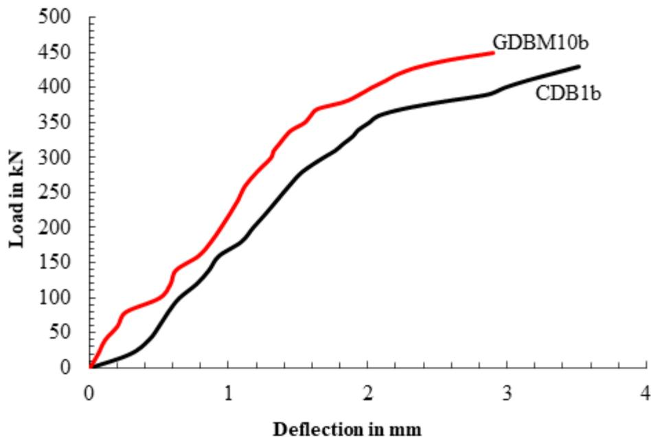
**Figure 9:** Load-deflection curves for the specimens CDB1b, & GDBM10b
