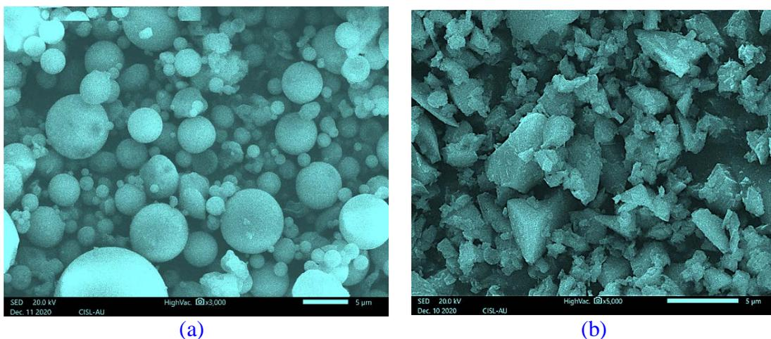
**Figure 2.** SEM Image a) Fly ash b) Alccofine.
