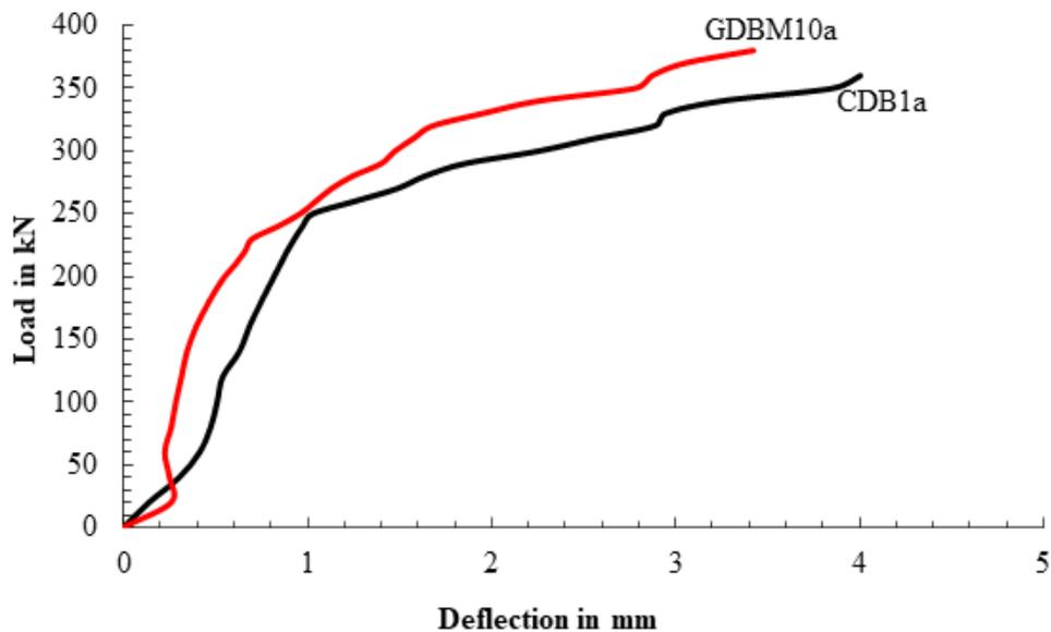
**Figure 8:** Load-deflection curves for the specimens CDB1a, & GDBM10a
