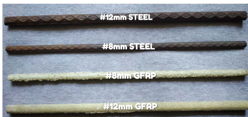
Figure 2: Steel and Sand-coated GFRP bars.
