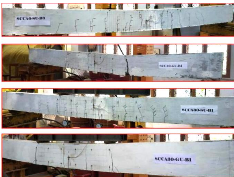
Figure 7: Crack Patterns of SCC Beams.
