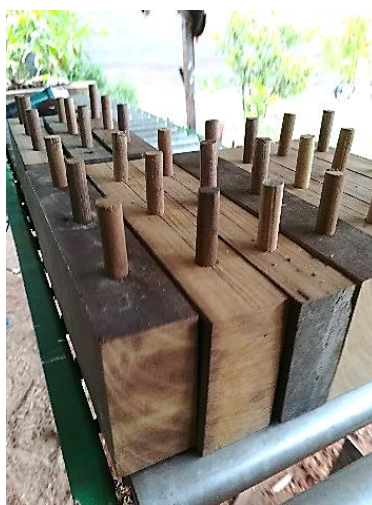
Figure 2: Withdrawal Block Test Specimens
