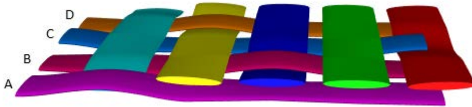
Figure 2: Cross-sectional view of Twill 4/1 weave structure by using TexGen software
