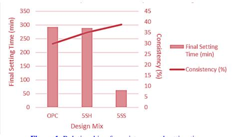
Figure 1: Relationship of consistency and setting time
