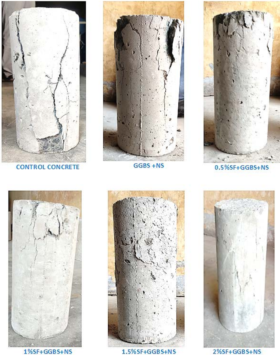
Figure 15: Failure Pattern of Cylinder specimens
