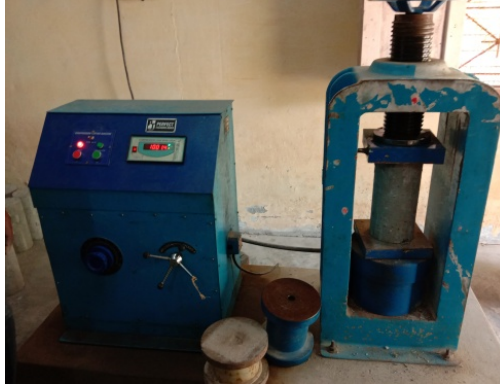
Figure 6: Cylinder Tested in Compressive Testing Machine
