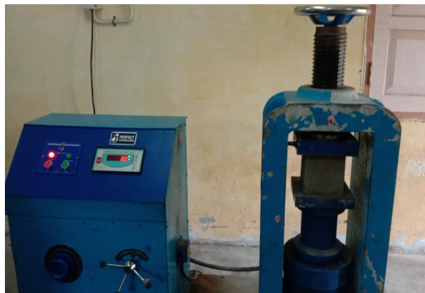
Figure 5: Cube Tested in Compressive Testing Machine
