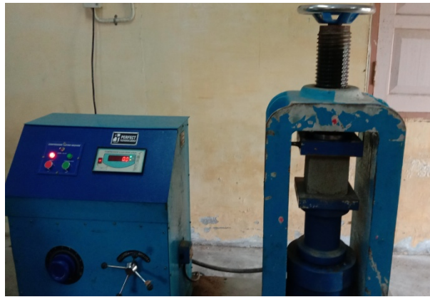
Figure 5: Cube Tested in Compressive Testing Machine
