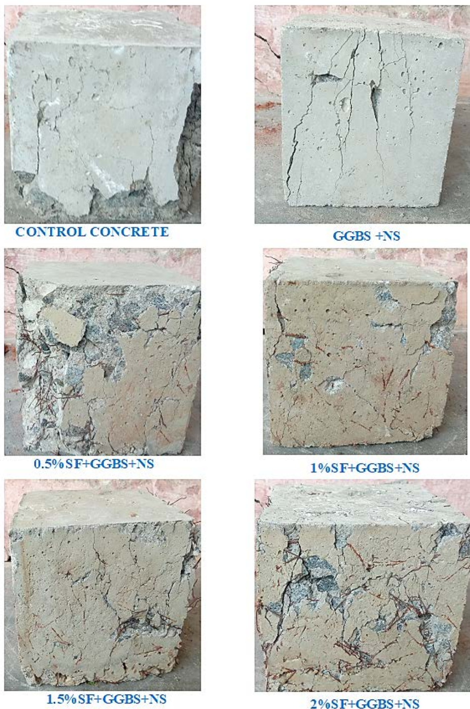
Figure 11: Failure Pattern of Cube specimens.
