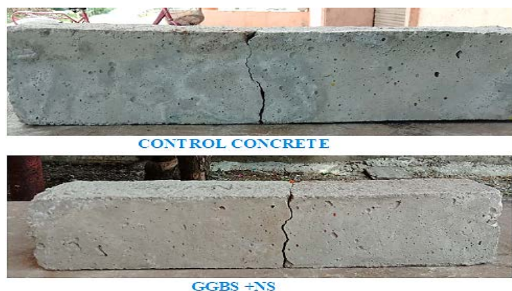
Figure 13: Failure pattern of prism specimens.
