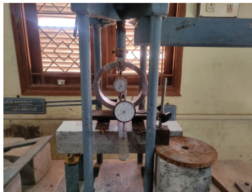
Figure 7: Test set-up for Flexural strength.
