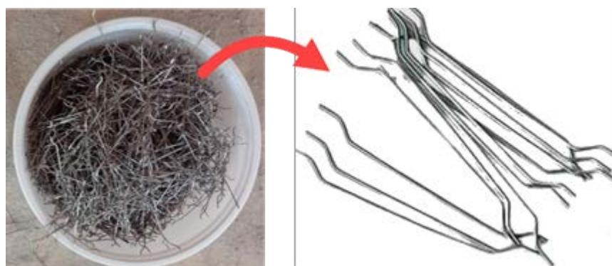
Figure 3: Hooked End Steel Fibres.
